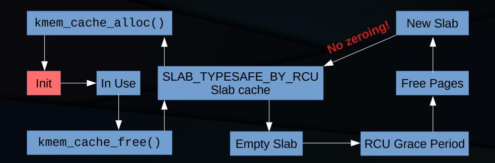
Without kmem\_cache\_zalloc(), "Init" cannot detect allocation from new slab!!!
