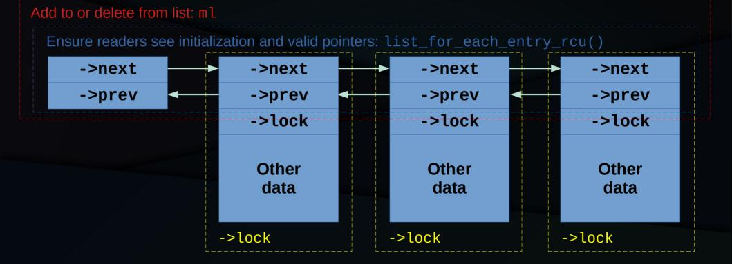
The ->lock protects "other data" and prevents the corresponding node from being removed.
